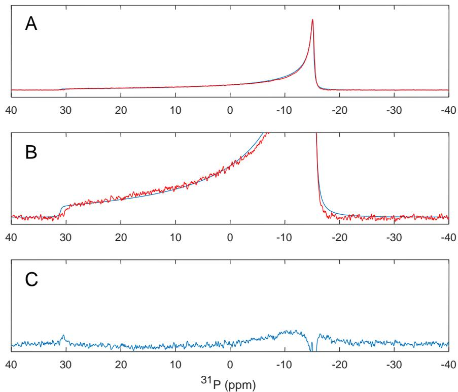
Figure S2. (A) Experimental (red) and simulated (blue) spectra of DPPC at 47°C with  $c/a=1.5$ . (B) Same as (A) with intensity multiplied by 10. (C) Residual intensity obtained after subtracting the experimental spectrum from the best-fit simulated one.
